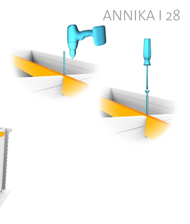
PLACE THE FIRST ROOFBOARD FLUSH WITH THE END OF THE PURLINS AND ATTACH WITH 6 SCREWS, 3 INTO EACH NEXT, SAW THE LAST BOARD TO MAKE IT FIT.
