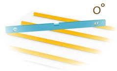
MAKE SURE THAT THE FOUNDATION IS INSTALLED ON A LEVEL SURFACE. CHECKING ALL DIRECTIONS, INCLUDING CORNER TO CORNER. 3%
