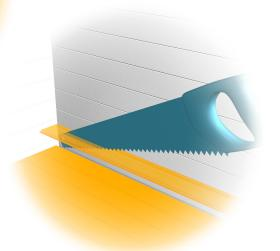
SAW THE BASEBOARDS AND ATTACH WITH NAILS AT EVERY 0,5 METERS.
