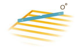
MAKE SURE THAT THE FOUNDATION IS INSTALLED ON A LEVEL SURFACE. CHECKING ALL DIRECTIONS, INCLUDING CORNER TO CORNER. 3% LAY OUT THE FOUNDATION BEAMS AND SQUARE IT BY MEASURING FROM CORNER TO CORNER.
